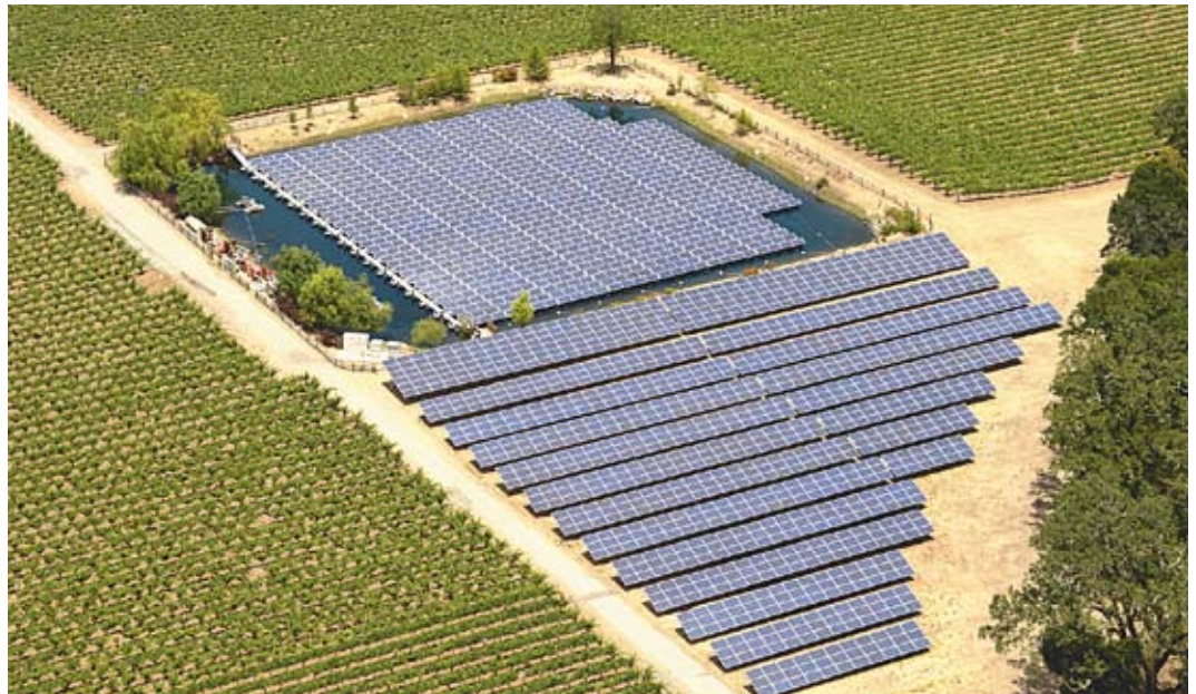
Sun Water Power 2 farm at Far Niente Winery near Oakville, California: in total the winery mounted more than 900 floating solar panels. A smaller amount of PV modules was installed on the ground.
