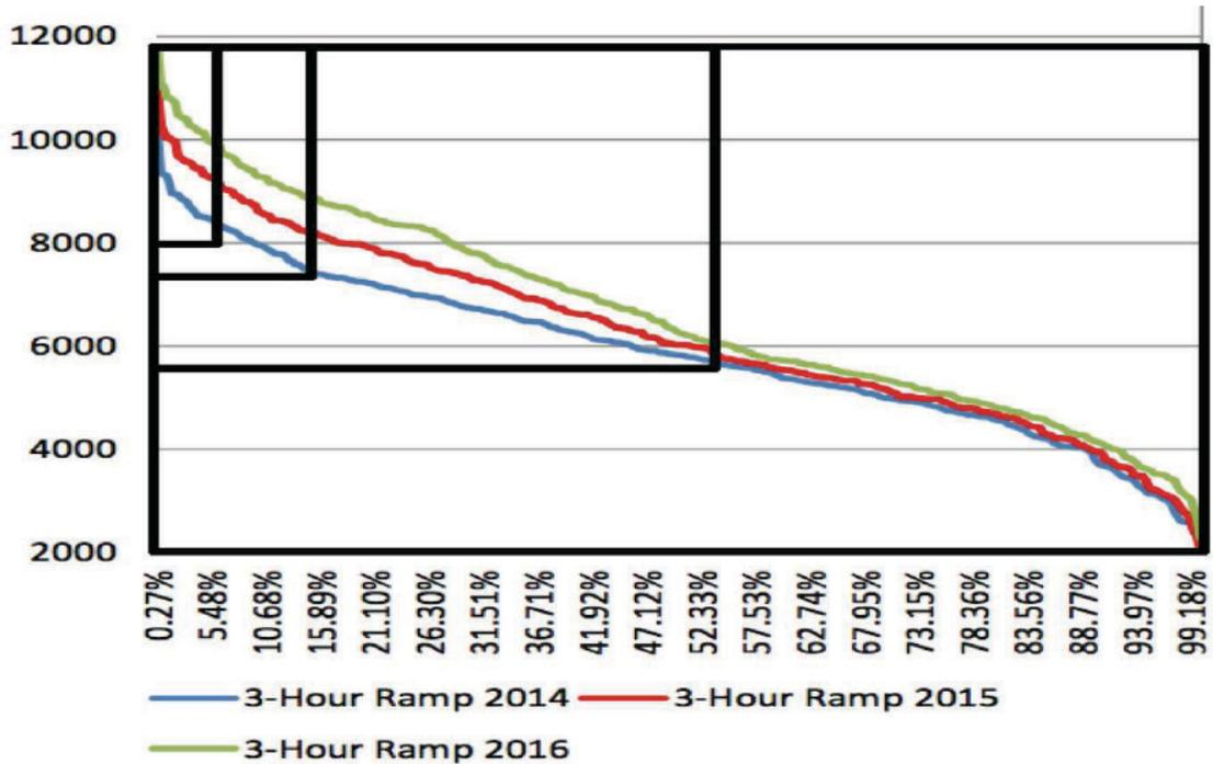
Available resources can be applied to whichever bucket they. Likewise, the same approach can be applied to other ramp mitigation options besides the three-hour continuous ramp illustrated in this example. As with the MCC, the buckets can be easily adjusted as the flexibility duration curve changes over time.
