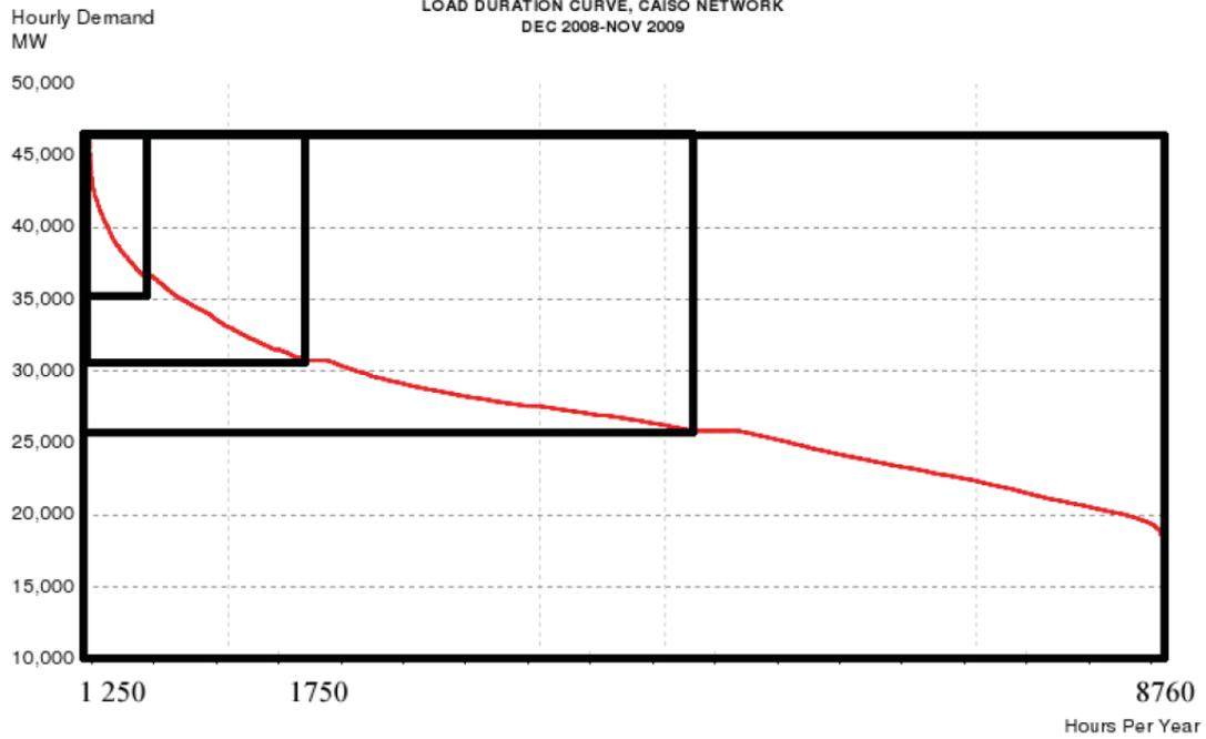
Figure 2. 3 Hour Flexibility Duration Curve with MCC-type buckets (Source: DECA/CAISO).
