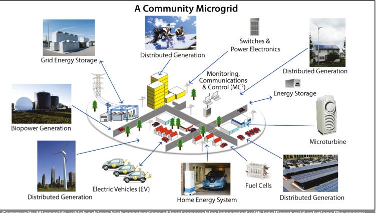
Community Microgrids, which achieve high penetrations of local renewables integrated with intelligent grid solutions like energy storage and advanced inverters, enable smarter, cleaner, and more resilient power systems.
