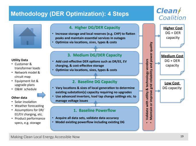
By starting with the Baseline DG Capacity first, then modeling a portfolio of distributed energy resources in combinations that leverage that Baseline DG Capacity, a utility can determine the optimal mix of local renewables and other DERs that result in the most cost-effective and resilient deployment for any given substation, the utility, and the community.
