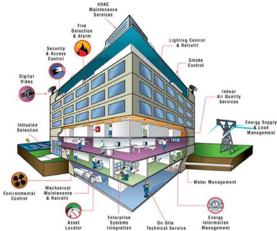
Figure 7: Building Automation System Segments
