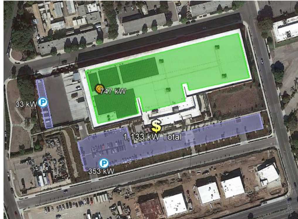
Solar Microgrid located at Direct Relief headquarters in Goleta, CA
