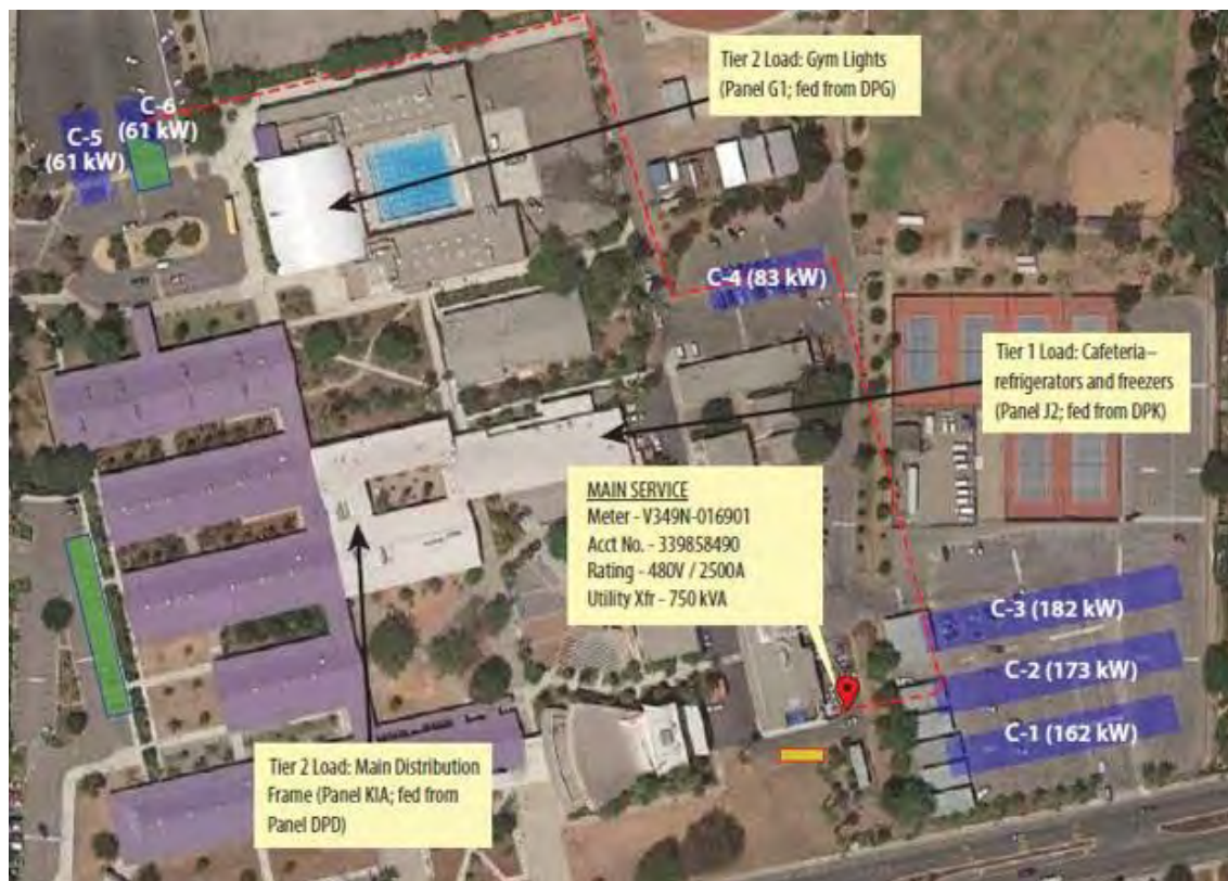
Figure 5: SMHS Solar Microgrid site layout
