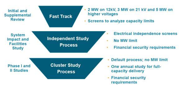
Customers requesting an Independent Study Process or a Cluster Study Process may apply for Full-Capacity Delivery. (Full-Capacity Delivery is the generating facility's ability to deliver its full output to the grid without constraints.)
