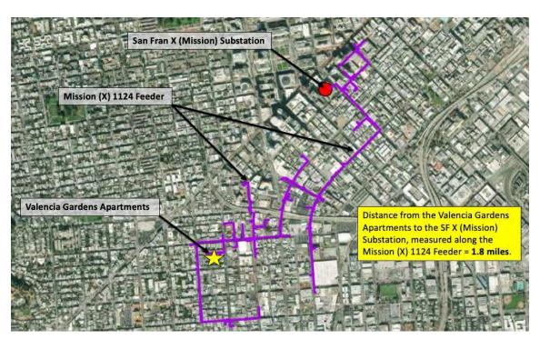
The following feeder map from PG&E also shows the Mission (X) 1124 Feeder from the San Fran X (Mission) substation. The feeder lines are colored according to their available capacity for adding solar, with green indicating more available capacity for adding solar onto the feeder and red indicating a higher probability of needing feeder upgrades for adding solar projects.
